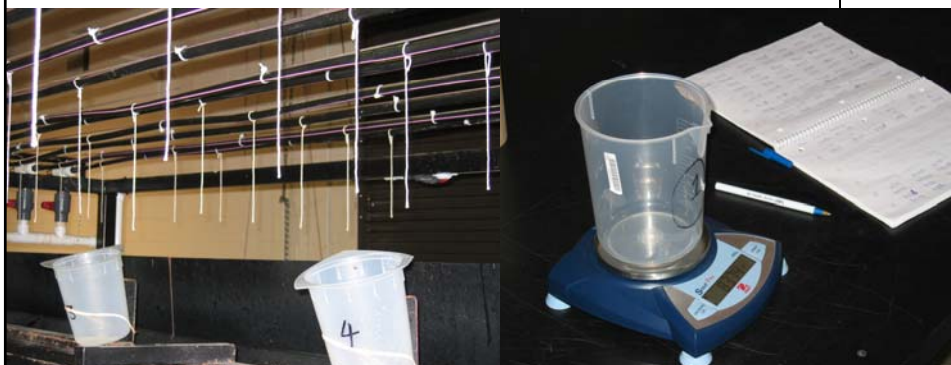
Weighing dry cans before sample event
